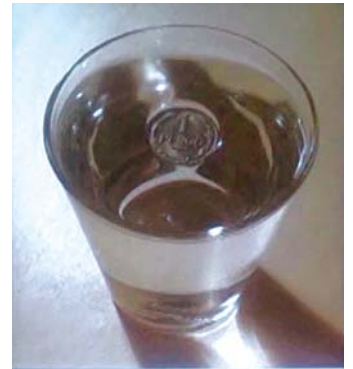
Fig. 16.1 Evidence of water's high surface tension
